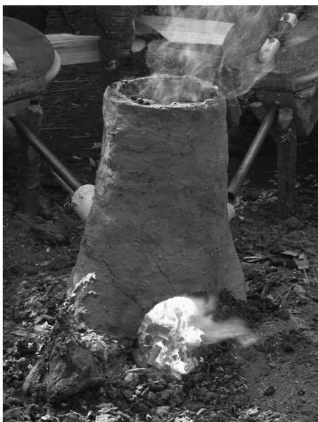
**A bloomery in action: Ottery iron ore produced plenty of slag and a small quantity of metallic iron. The experiment made clear the potential for iron production using local ore.**
